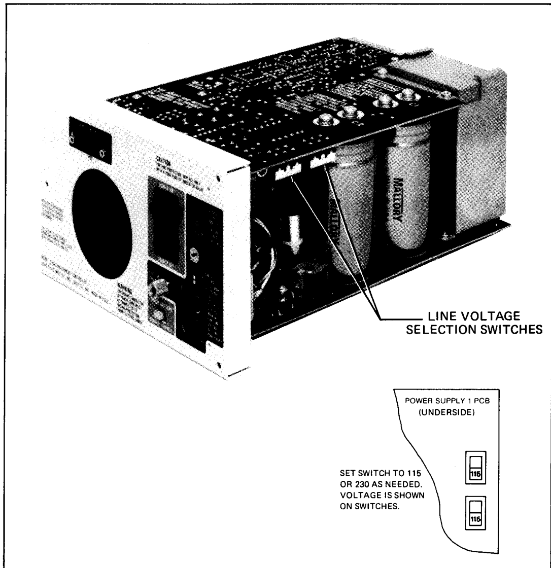
Figure 2-1. Power Voltage Range Selection
